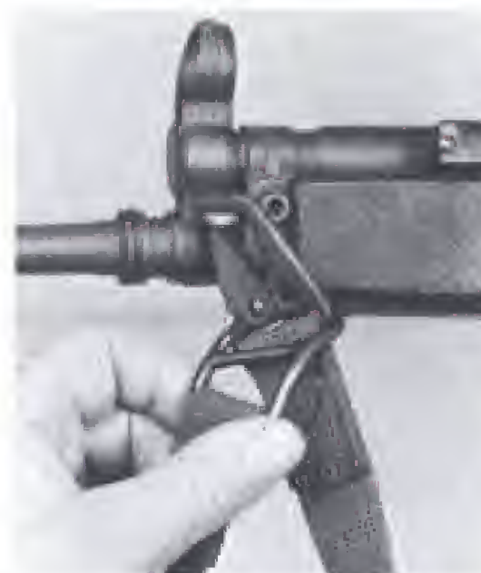
Fig. 39 Pulling the double loop over the carbine hook
